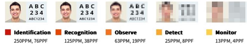
The FoV image value is calculated based on the maximum resolution supported by the camera. The required minimum pixel density would vary depending on application, and should be used as a guideline only. Also, the level of detail may vary from type of video analytics software used.
